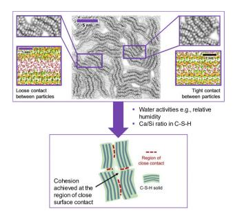
Fig. 2 Schematic picture of the nanoscale structure of the CSH gel (center). In the top-left and -right, the magnifications show two possible interparticle interfaces: a loose (left) and tight (right) contact. The close contact among CSH particles contributed to the strength of the CSH pellet as seen in the developed case in ref. 8 (reproduced from ref. 8 and 9 with permission from Elsevier, copyright 2022).
