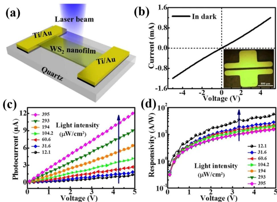
Fig. 15 (a) Lateral device schematic structure of the photodetector, (b) *I*–*V* characteristics measured in the voltage range of the photodetector, (c) responsivity of the device with different light intensities and (d) responsivity with respect to applied bias at different illumination intensities. Reprinted with permission of ref. 160, Copyright of Nature 2016.
