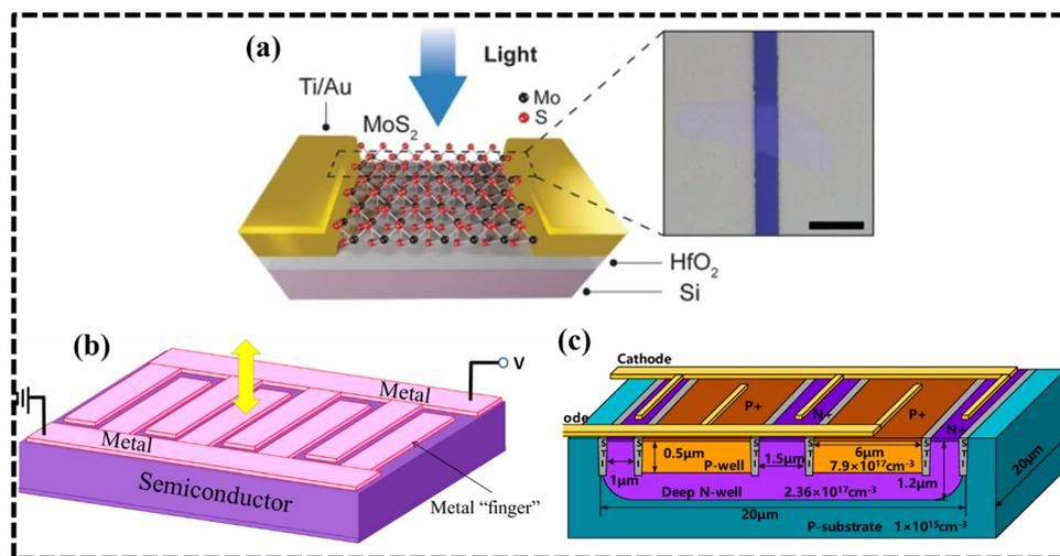
Fig. 12 (a) High responsivity in MoS<sub>2</sub> phototransistors based on charge trapping HfO<sub>2</sub> dielectrics,<sup>155</sup> (b) avalanche photo diode,<sup>156</sup> and (c) MoS<sub>2</sub> phototransistors. Reprinted with permission from ref. 157.
