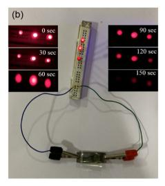
Fig. 8 (a) Ragone plot of NiCo-CH-180//AC compared with the literature on devices with similar electrode materials and (b) photograph of a device to light three red LEDs.
