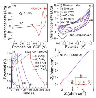
Fig. 6 (a) CV curve of the negative (AC) and positive (NiCo-CH-180) electrode at 10 mV s<sup>-1</sup> in a three-electrode set up. (b) CV curves for the ASC at various scan rates (10-100 mV s), (c) GCD curves at different current densities (2-10 A g<sup>-1</sup>), and (d) Nyquist plot of the NiCo-CH-180// AC ASC (two-electrode device)
