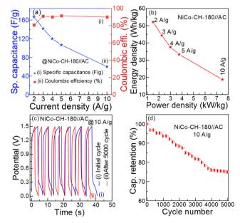
Fig. 7 (a) Specific capacitance and coulombic efficiency of NiCo-CH-180//AC ASC at different current densities (2-10 A g<sup>-1</sup>), (b) Ragone plot (ED vs. PD), (c) initial and after 5000 charge-discharge curves, and (d) capacitance retention performance up to 5000 charge-discharge cycles at 10 A  $\rm g^{-1}$  current density of the NiCo-CH-180//AC ASC.
