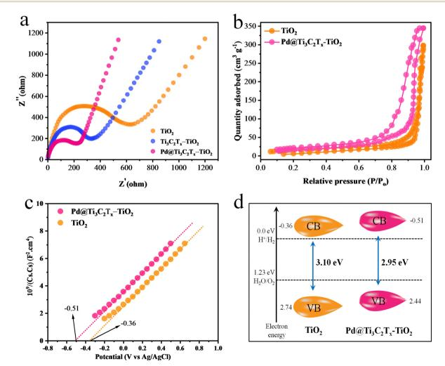
Fig. 8 (a) EIS results of  $TiO_2$ ,  $Ti_3C_2T_x-TiO_2$  and  $Pd@Ti_3C_2T_x-TiO_2$ . (b) BET results, (c) Mott-Schottky and (d) calculated band positions of  $TiO_2$  and  $Pd@Ti_3C_2T_x-TiO_2$ .
