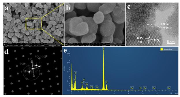
Fig. 4 SEM images at (a) 1 μm and (b) 200 nm, (c) HR-TEM, (d) TEM diffraction pattern, and (e) EDX analysis of Pd@Ti<sub>3</sub>C<sub>2</sub>T<sub>x</sub>-TiO<sub>2</sub>.
