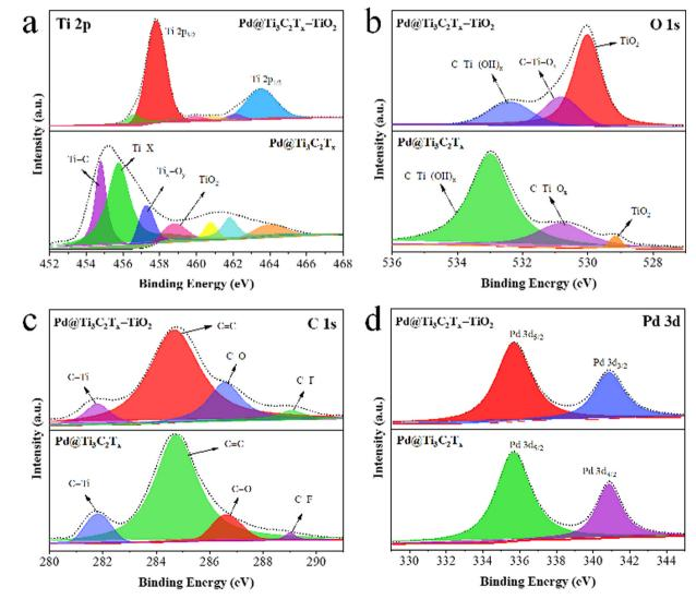
Fig. 6 XPS results of Pd@Ti $_3$ C $_2$ T $_x$  and Pd@Ti $_3$ C $_2$ T $_x$ -TiO $_2$ : (a) Ti 2p, (b) O 1s, (c) C 1s, and (d) Pd 3d
