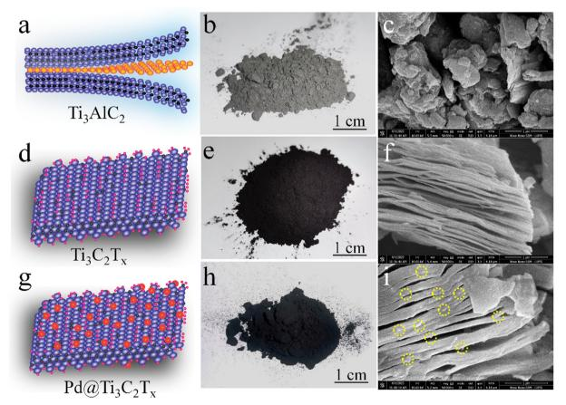
Fig. 3 (a) Schematic illustration, (b) digital photograph, and (c) SEM image of MAX ( $T_{13}AlC_2$ ). (d) Schematic illustration, (e) digital photograph, (f) SEM image of MXene ( $T_{13}C_2T_x$ ). (g) Schematic illustration, (h) digital photograph, and (i) SEM image of Pd@MXene ( $Pd@T_{13}C_2T_x$ ).
