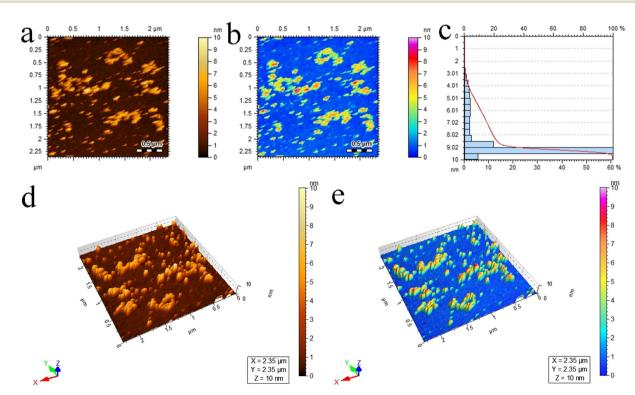
Fig. 5 AFM results of Pd@Ti<sub>3</sub>C<sub>2</sub>T<sub>x</sub>-TiO<sub>2</sub> photocatalysts: (a) and (b) 2D-tapping modes, (c) size distribution and (d) and (e) 3D images.
