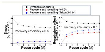
Fig. 3 Smog (SG) and respiratory effect (RP) of synthesis of AuNPs and two recovery/recycling processes with varying number of reuse cycles (#). The recovery efficiency was set to 0.6.
