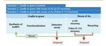
Fig. 1 System boundary of AuNP-based sensing with three different scenarios: control (without reuse) and two Au nano-waste reuse strategies.
