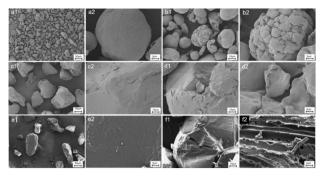
Fig. 1 SEM images of microplastics before and after UV weathering, (a1 and a2) pristine PE; (b1 and b2) PE weathered for 120 days; (c1 and c2) pristine PS; (d1 and d2) PS weathered for 60 days; (e1 and e2) pristine PBAT; (f1 and f2) PBAT weathered for 120 days.
