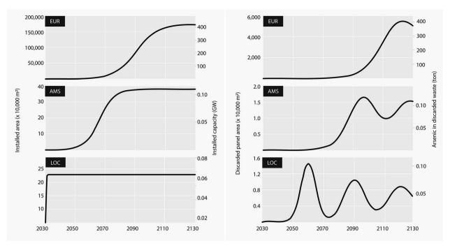
Projected III-V/Si PV demand (left) and discarded materials (right) for the three scales
