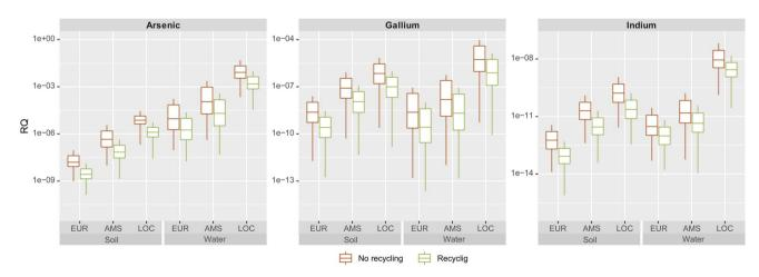
Fig. 4 Risk quotients for arsenic, gallium and indium in soil and freshwater compartments in all scales, with and without recycling.
