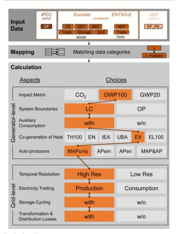
**Fig. 3** Grid EF calculation methodology, grouped into the layers input data, mapping and calculation. The calculation layer consists of two parts, comprising generator-level and grid-level calculations. The boxes highlighted in orange illustrate one example set of choices.
