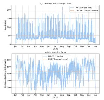
Fig. 9 (a) Electrical grid load profile of the Battery Lab Factory in Braunschweig (BLB) and (b) corresponding grid EF for Germany in 2021. Both high (15 minute) and low (annual) resolutions are presented (HR, LR). The recommended grid EF configuration (cf. Section 5.2.1) is applied.
