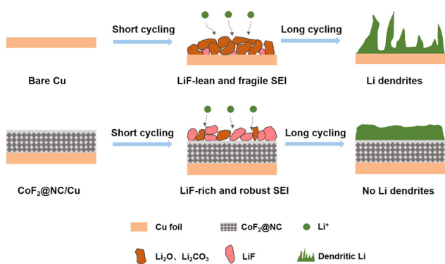
Fig. 7 Schematic illustration of the Li stripping/plating cycling on (a) bare Cu and (b) \text{CoF}_2@NC/Cu current collectors.
