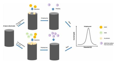
Fig. 16 The total arsenic concentration measured by deposition at -1.3 V while the As(III) measured at -0.9 V on gold macroelectrodes based on the underpotential deposition (UPD) of As ad-atoms<sup>131</sup> (reprinted from ref. 131; Copyright (2022), with permission from Elsevier).
