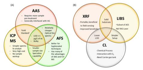
Fig. 4 (A) Illustration of spectroscopic methods: AAS, ICP MS and AFS<sup>11</sup> (reproduced from ref. 11 with permission from the Royal Society of Chemistry, Copyright [2015]), (B) XRF, LIBS and CL for detection of arsenic.
