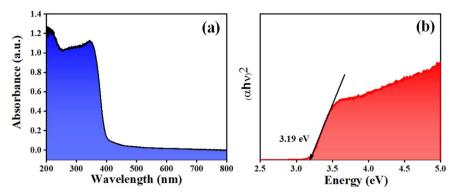
Fig. 3 (a) DRS of BaTiO<sub>3</sub>, (b) Tauc's plot for energy band gap.
