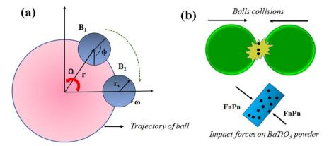
Fig. 10 (a) Trajectory of balls in planetary motion, (b) mechanics of balls for generating piezocatalysis in BaTiO<sub>3</sub> powder.
