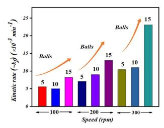
Fig. 6 Kinetic rate (kf) in min<sup>-1</sup> of MB dye degradation using 5, 10, and 15 balls at 100, 200, and 300 rpm.
