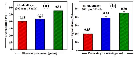
Fig. 7 Degradation of  $\sim 5$  mg L $^{-1}$  concentrated MB dye at 200 rpm milling speed using 0.15, 0.20, and 0.30 grams of BaTiO $_3$  powder for (a) 30 mL and (b) 50 mL.
