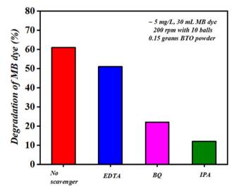
Fig. 12 Scavenger test for degradation of MB dye.
