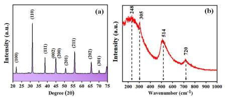
Fig. 1 Synthesized BaTiO<sub>3</sub> (a) XRD pattern, (b) Raman spectrum.
