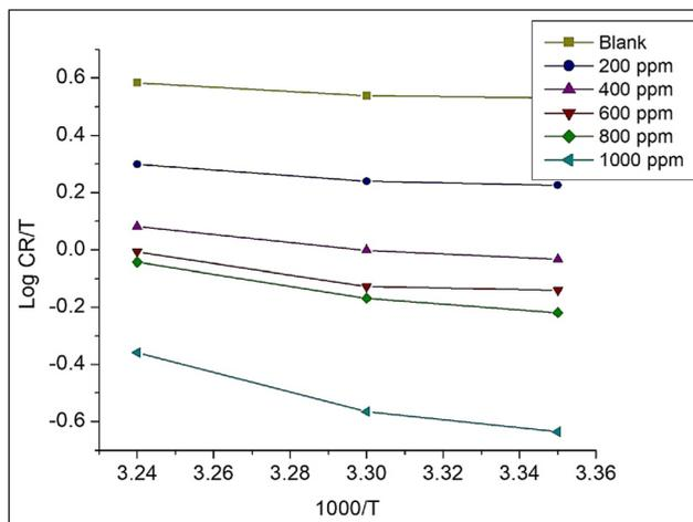
Fig. 9 Plot of log CR/T versus 1000/T for Co<sub>3</sub>O<sub>4</sub>@PPy NCs.
