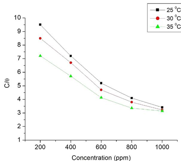
Fig. 10 Langmuir adsorption isotherm ( $C/\theta$ ) versus concentration of Co<sub>3</sub>O<sub>4</sub>@PPy NCs at 25, 30, and 35 °C.
