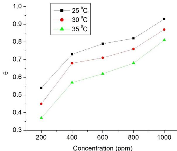
Fig. 11 Henry adsorption isotherm ( $\theta$ ) versus concentration (ppm) of Co<sub>3</sub>O<sub>4</sub>@PPy NCs at 25, 30, and 35 °C.
