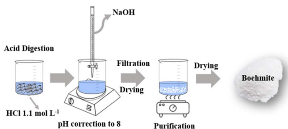
Fig. 1 Scheme of the synthetic route used to obtain boehmite. (Adapted from ref. 23).
