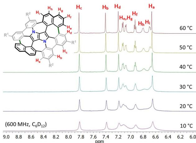
**Fig. 3** Variable temperature <sup>1</sup>H-NMR spectrum of the molecular N-doped saddle **8** in the aromatic region (from 6.0 to 9.0 ppm) recorded in cyclohexane-*d*<sub>12</sub> (600 MHz, 10–60 °C).
