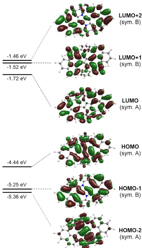
Fig. 7 Selected Kohn-Sham molecular orbitals of the truncated molecular saddle **8H** and their energy levels calculated with the aid of DFT at the B3LYP/cc-pVDZ level of theory. An isovalue of 0.02 was used for the depiction of each MO, the view corresponds to the top face of the molecule.
