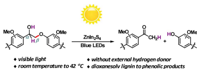
Fig. 8 Visible-light-driven fragmentation of lignin \beta -O-4 models and dioxanesolv lignin. Adapted from ref. 19 with permission. Copyright 2017 American Chemical Society.
