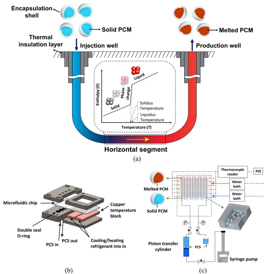
**Fig. 3** Lab-on-a-chip analysis of processes relevant to geothermal energy. A closed-loop geothermal system (a) is a closed system, and can benefit from specialized working fluids. The work highlighted here employs LoC methods (b and c) to assess the potential for a microencapsulated phase change slurry as a working fluid, with testing at temperatures, pressures and shear-rates relevant to large scale operations. Reprinted with permission from ref. 121 copyright 2021 American Chemical Society.
