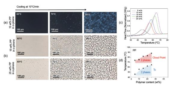
Fig. 2 (a) Polarized and (b) non-polarized optical microscopy cloud point (CP) measurements; (c) crystallization ( $T_c$ ) measurement by DSC temperatures for PP in α-pinene; and (d) corresponding phase diagram.
