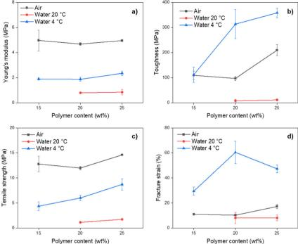
Fig. 5 Mechanical properties of pure PP membranes prepared with 15, 20, and 25 wt% polymer contents in α-pinene and quenched in air at room temperature, water at 20 °C, and water at 4 °C. (a) Young's modulus, (b) toughness, (c) tensile strength and (d) fracture strain.
