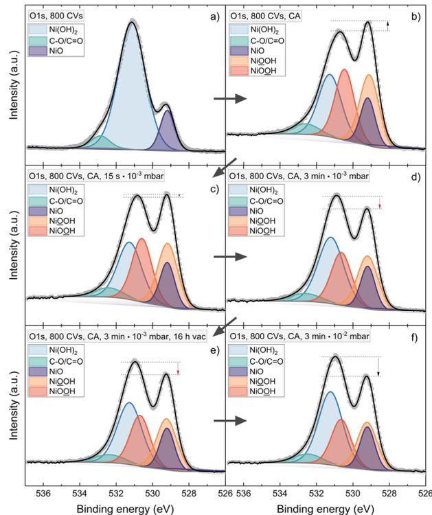
**Fig. 6** XPS spectra of the O1s line of a 120 nm NiO thin film with an activation treatment of 800 CVs. (a) Situation before *ex situ* treatments. After *ex situ* chronoamperometry (CA) at 1.50 V vs. RHE (b), the sample was exposed *in vacuo* to increasing amounts of water vapor (c, d and f). The fitting shows the decrease of NiOOH in contact with water. The stability in vacuum is shown in e) compared to d).
