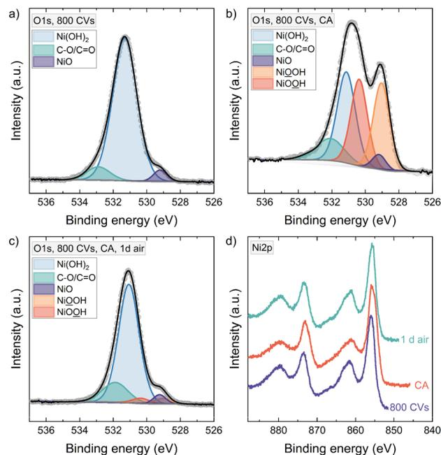
**Fig. 4** XPS spectra of the fitted O1s and Ni2p regions of a 6 nm NiO thin film after an activation treatment of 800 CVs. a) with 800 CVs, NiO was almost completely transformed to Ni(OH)<sub>2</sub>. b) after CA at 1.55 V vs. RHE, NiOOH is detected. c) Keeping the portion of the NiO peak constant in the fitting of the O1s region, little NiOOH is needed to fit the spectrum after storing the sample for one day in atmospheric conditions. d) Ni2p lines after 800 CVs, CA, and storage in air.
