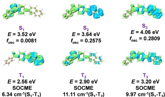
**Fig. 3** Iso-surface maps of the electron-hole density difference of **6**'s  $S_n$  and  $T_n$  states calculated in Gaussian 16 by TD-DFT/B3LYP/6-31G(d,p), where blue and green iso-surfaces correspond to hole and electron distributions, respectively, and SOCME values calculated on ORCA 4.2.1 by TD-DFT/B3LYP/def2-TZVP(-f).
