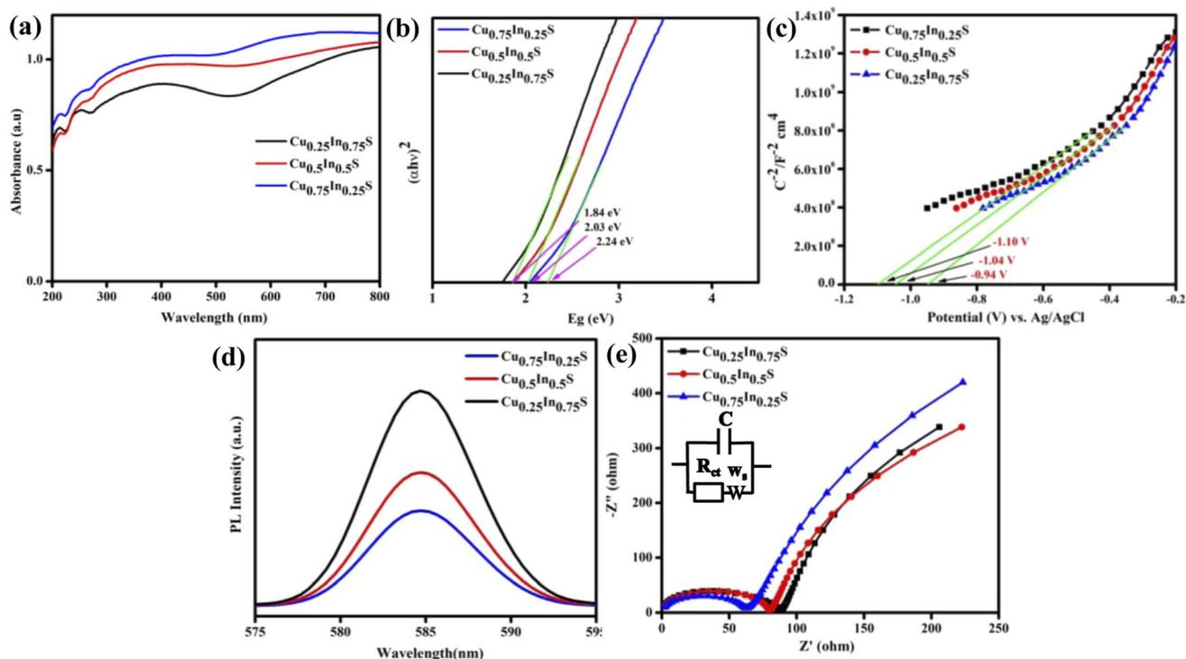
Fig. 2 Optoelectronic study of  $\text{Cu}_{0.25}\text{In}_{0.75}\text{S}$  (black line),  $\text{Cu}_{0.5}\text{In}_{0.5}\text{S}$  (red line), and  $\text{Cu}_{0.75}\text{In}_{0.25}\text{S}$  (blue line) QDs: (a) UV-Vis DRS spectra, (b) Tauc plot, (c) the  $M-S$  plot over a frequency of 1000 Hz in 0.1 M  $\text{Na}_2\text{SO}_4$ , (d) PL spectra, and (e) the EIS plot.
