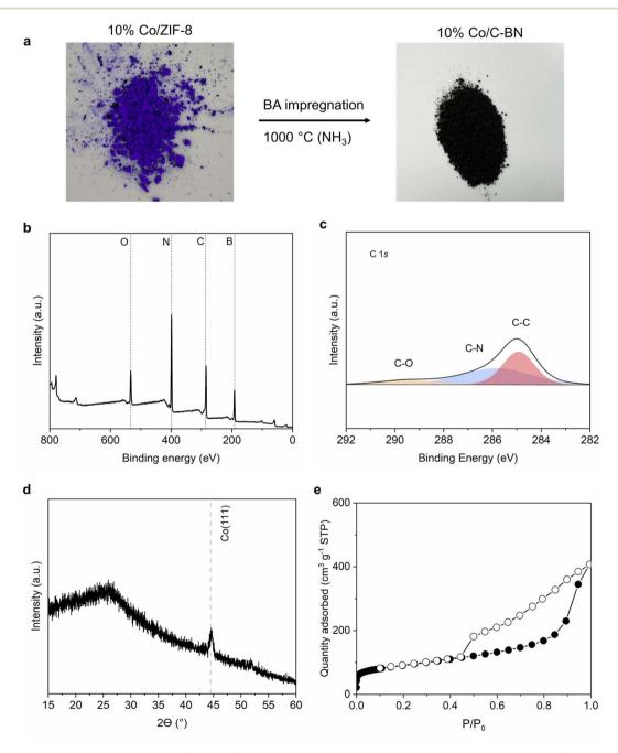
Fig. 8 Synthesis and characterisation of 10% Co/C-BN. (a) Synthesis process of 10% Co/C-BN; (b) XPS survey spectra; (c) high resolution XPS in the region of C 1s; (d) XRD patterns; (e) N<sub>2</sub> sorption isotherms at 77 K.
