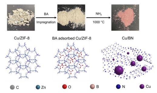
Scheme 1 Schematic representation of Cu/BN synthesis
