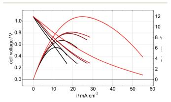
Fig. 4 LSV curves for a cell with a Ni–Co–CGO anode measured in 3%  $H_2O/H_2$  at 750 °C (reference conditions) after operation in various  $CH_4/CO_2$  atmospheres at 750 °C for 15 minutes each. The LSV curves (left axis) are plotted together with the calculated power curves (right axis).
