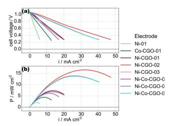
Fig. 3 Initial LSV (a) and power density curves (b) of all the tested cells, measured in 3% H<sub>2</sub>O/H<sub>2</sub> at 750 °C
