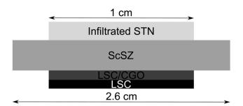
Fig. 1 Schematic representation of the fuel cell assembly tested in these studies. Notably, the thickness of these layers is not to scale.
