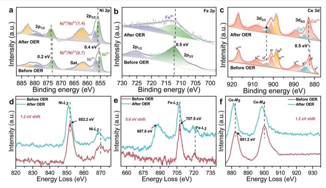
Fig. 6 High-resolution XPS spectra of CeO<sub>2</sub>@NiFe-MOFs before and after the OER: (a) Ni 2p, (b) Fe 2p, and (c) Ce 3d. (d-f) The corresponding EELS spectra of CeO<sub>2</sub>@NiFe-MOFs before and after the OER: (d) Ni-L, (e) Fe-L, the peak at 687.8 eV is attributed to F-K (Fig. S31†), and (f) Ce-M.
