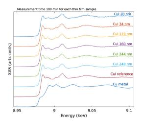
Fig. 9 XANES spectra of the Cu K edge of the Cul thin films and references.
