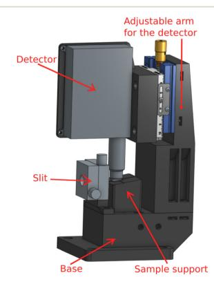
**Fig. 2** The fluorescence mode setup for measuring thin films, consisting of a base, slit, sample support, detector, and an adjustable arm for the detector.
