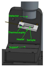
Fig. 6 An illustration of sample annealing setup.
