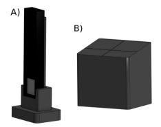
Fig. 3 The two pieces for alignment: (A) vertical support for the Minipix-detector, (B) support for the sample where the sample positioning is at 10° angle. The sample will be centered at the crosshair position.
