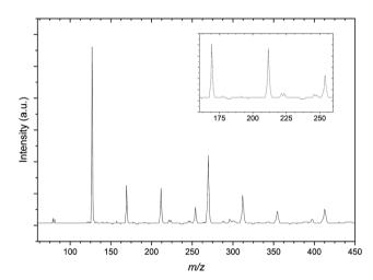
Fig. 3 Mass spectrum resulting from the CH<sub>3</sub>I:C<sub>3</sub>H<sub>6</sub>:Ar gas mixture. The spectrum shows mass peaks resulting from the bare Br- anions and propene complexes with I<sup>-</sup>. Inset: Highlighted the peaks at 169, 211 and 254 m/z assigned to the  $I^- \cdots (C_3 H_6)_n$  (n = 1-3) complexes.
