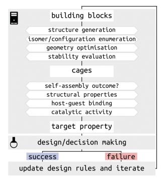
Fig. 1 Schematic of the steps and challenges toward MOC design and assisting experimental decision making. The broader process of MOC design will be an iterative consideration of successes and failures, which update our design principles.
