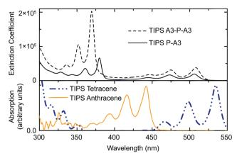
Fig. 5 UV-Vis Absorption spectra of TIPS anthracene, TIPS tetracene, TIPS P-A3, and TIPS A3-P-A3. The absorption for TIPS P-A3 is red-shifted compared to TIPS anthracene, but blue-shifted to TIPS tetracene.
