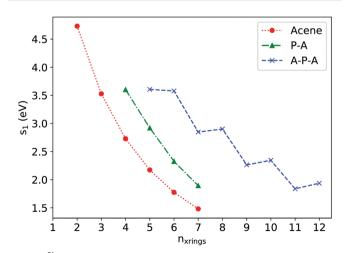
Fig. 4  $\varepsilon^{S1}$  as a function of  $n_{xrings}$  for acenes, P-A and A-P-A as determined via TDDFT at the (OT)-LC-ωHPBE/Def2TZVP level of theory.
