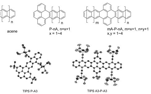
Fig. 1 Molecular structures and their abbreviations used throughout this study. (Top) Molecules used in theoretical calculations (bottom) thermal ellipsoids of pyrenoanthracene (TIPS P-A3) and pyrenodianthracene (TIPS A3-P-A3).
