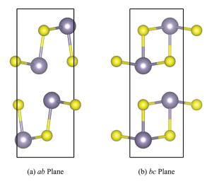
Fig. 1 Structure of *Pnma* SnS shown through the *ab* (a) and *bc* (b) planes, illustrating the layering along the *b* axis and the anisotropic chemical bonding along the perpendicular in-plane *a* and *c* axes. S and Sn atoms are shown in yellow and grey, respectively. These images were prepared using the VESTA software (ref. 50).
