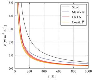
Fig. 10 Predicted averaged thermal conductivity  $\kappa_{\rm ave}$  of SnSe (black) and the  $\kappa_{\rm ave}$  of Sn(S<sub>0.1875</sub>Se<sub>0.8125</sub>) obtained using the three models considered in this section: the mass-variance model (blue), the CRTA model defined in eqn (3) and (4) with an interpolated lifetime  $\tau^{\rm CRTA}$  (red), and the model defined in eqn (8) with the interaction strengths  $P_{\lambda}$  replaced by an interpolated constant  $\tilde{P}$  (orange).
