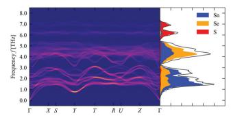
Fig. 6 Unfolded dispersion and atom-projected density of states (PDoS) of  $Sn(S_{0.1875}Se_{0.8125})$ . The colour scale in the unfolded dispersion represents the spectral weight and runs from blue (low weight) to yellow (high
