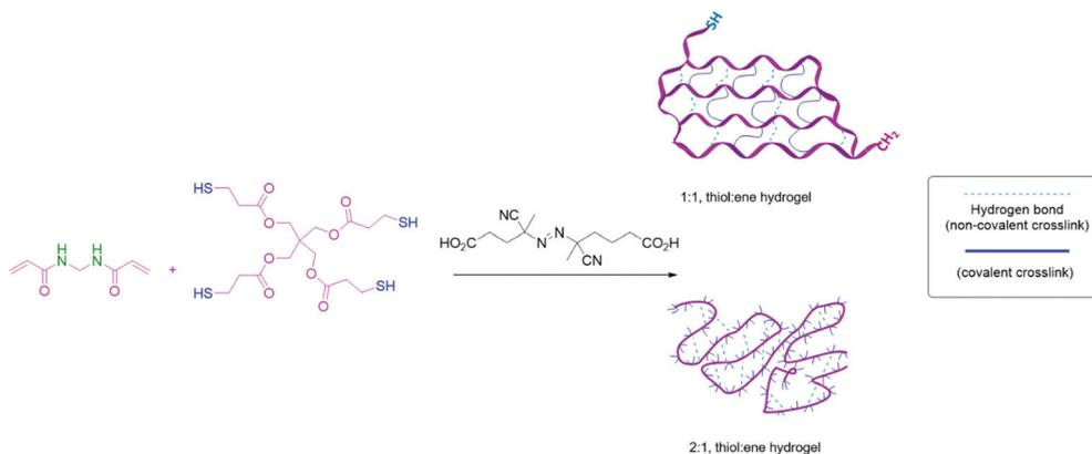
Fig. 1 The copolymerization of *N,N*-methylene bis(acrylamide) with pentaerythritol tetrakis(3-mercaptopropionate) to form controlled and tunable hydrogels.
