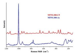
Fig. 11 Raman spectra of MFM-300(Sc) after 5 cycles of  $H_2S$  (red) and as synthesised (blue). The peaks observed in the  $350-520~{\rm cm}^{-1}$  region are associated to the S–S stretching vibrations modes of several polysulphides with various chain lengths. Reprinted with permission from ref. 70. Copyright (2020) American Chemical Society.
