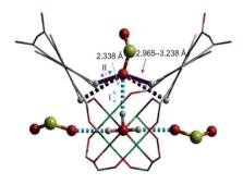
**Fig. 2** Preferred binding sites for SO<sub>2</sub> molecules inside MFM-300(Al) determined by *in situ* PXRD. (I) Moderated hydrogen bond. (II) Weak hydrogen bond. Reprinted (adapted) with permission from ref. 37a. Copyright (2012) Springer Nature.
