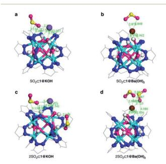
Fig. 6 DFT structure minimization of molecular configuration of one (a and b) and two (c and d) adsorbed  $SO_2$  molecules on 1@KOH (left) and  $1@Ba(OH)_2$  (right) materials. For sake of clarity, only the region around the metal cluster is shown. Ni (cyan); K (purple); Ba (wine); C (grey); N (blue); O (magenta); H (white); S (yellow). Reprinted (adapted) with permission from ref. 45. Copyright (2017) Springer Nature.
