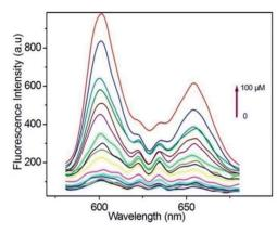
Fig. 14 Fluorescence spectra of porphyrin ligand (10  $\mu$ M) in BBS butter (pH = 7.40, 20 mM) after titration with HS $^-$  from 0–100  $\mu$ M,  $\lambda_{ex}=419$ . Reprinted with permission from ref. 94. Copyright (2014) American Chemical Society.
