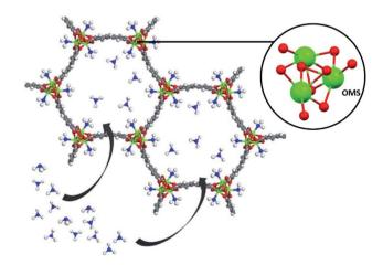
Fig. 18 Atomic structure of  $M_2$ (dobpdc) complexes with one-dimensional hexagonal channels. It is possible to observe that each coordinatively unsaturated metal site points towards the channel Reprinted (adapted) with permission from ref. 109. Copyright (2020) John Wiley & Sons.
