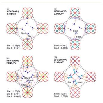
Fig. 20 Preferential  $ND_3$  binding sites in MFM-300(M) family (M = Cr, Fe,  $V^{3+}$ ,  $V^{4+}$ ) determined by NPD at 10 K. Views along c axis. Reprinted with permission from ref. 111. Copyright (2021) American Chemical Society.
