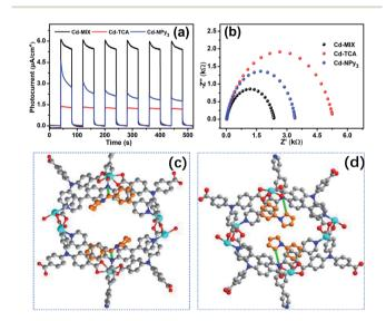
Fig. 6 Photocurrent tests (a) and EIS plots (b) of Cd-MIX, Cd-TCA, and Cd-NPy<sub>3</sub> under the same conditions, showing the superiority of Cd-MIX over the others. The interaction patterns between the embedded substrates (1c and 1a) and active sites in the channels of 1c@Cd-MIX (c) and 1a@Cd-MIX (d).
