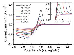
Fig. 3 Cyclic voltammograms of the ORR and OER on Au at various scan rates in  $\rm O_2$ -saturated 0.1 M TBAClO<sub>4</sub>/0.01 M Ca(ClO<sub>4</sub>)<sub>2</sub>/DMSO. The inset shows the enlarged positive sweeps to show the OER features at lower scan rates. Variable scan rate voltammograms were collected after 150 cycles at 100 mV s $^{-1}$  within the same potential range.
