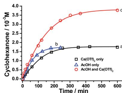
Fig. 5 Time trace for cyclohexane oxidation by  $[\text{Pr}_4\text{N}][\text{RuO}_4]$  (0.01 M) in  $\text{CH}_3\text{CN}$  at 23 °C in the presence of (a) 1 equiv.  $\text{Ca}^{2+}$ , (b) 12 mol equiv. of  $\text{AcOH}$  and (c) 1 mol equiv.  $\text{Ca}^{2+}$  + 12 mol equiv.  $\text{AcOH}$ .
