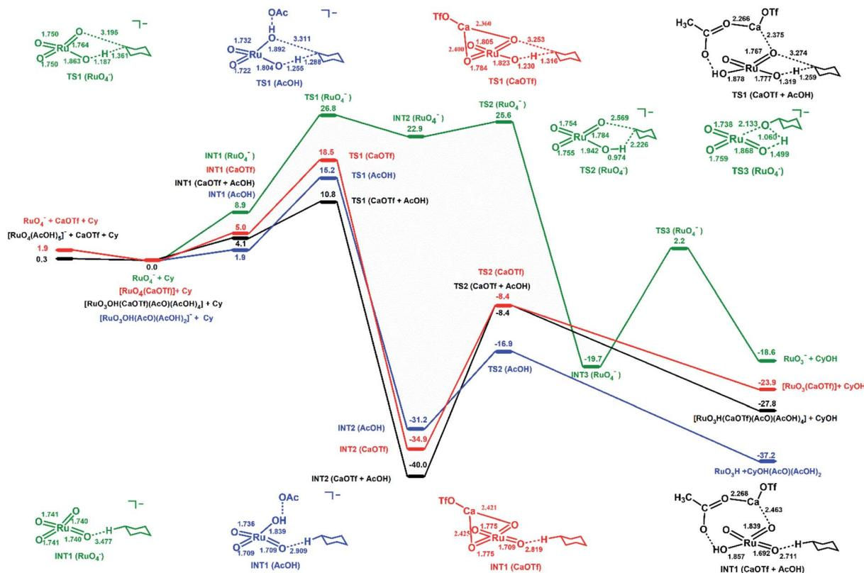
Fig. 7 PESs for cyclohexane oxidation by  $[\text{RuO}_4]^-/[\text{RuO}_4(\text{AcOH})]^-/[\text{RuO}_4(\text{CaOTf})]/[\text{RuO}_4(\text{AcOH})(\text{CaOTf})]$  at the B3LYP level using LanL2TZ(f) basis set (Ru) and 6-311++G(d,p) basis set (non-metals). Relative 298 K Gibbs free energies in acetonitrile are given in  $\text{kcal mol}^{-1}$ . Not all acetic acid molecules are shown for simplicity.
