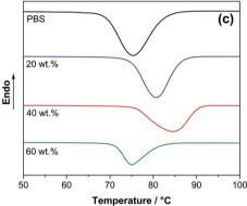
Fig. 3 DSC (a) first heating curves, (b) second heating curves, and (b) cooling curve for PBS and 20, 40, and 60 wt% PBS/SCG composites.
