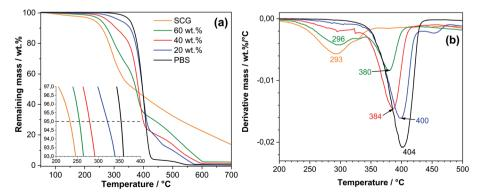
(a) TGA thermogram and (b) first derivative TGA curves of PBS and PBS/SCG composites.
