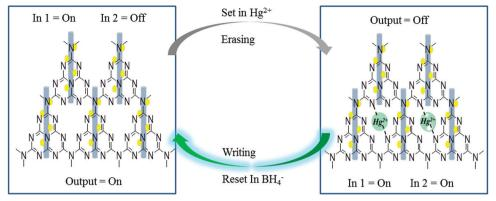
Scheme 2 Probable mechanistic pathway for the grafting of Hg<sup>2+</sup> with g-C<sub>3</sub>N<sub>4</sub>/Ag/ZnWO<sub>4</sub> and further reduction of Hg<sup>2+</sup> by NaBH<sub>4</sub>, correlated with Implication Logic Gate.
