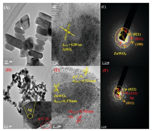
Fig. 3 (A)–(C) Show the TEM, HR-TEM, and SAED patterns of  $ZnWO_4$ , respectively, and (D)–(F) are TEM, HR-TEM, and SAED patterns of  $g-C_3N_4/Ag/$ ZnWO<sub>4</sub>, respectively.
