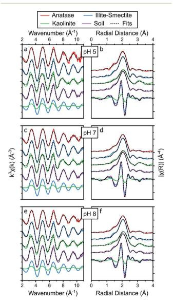
Fig. 5 Summary of the Sr K-edge EXAFS (a, c and e) and the respective Fourier transform (b, d and f) of the adsorption samples at pH 5 (a, b), 7 (c, d) and 8 (e, f), including the results from the holistic fitting strategy (black dotted lines, Table 2) and the respective contribution of the EXAFS and FT of Sr adsorbed to illite-smectite and kaolinite to the fits to the EXAFS of Sr adsorbed to the soil samples at the bottom of each panel.
