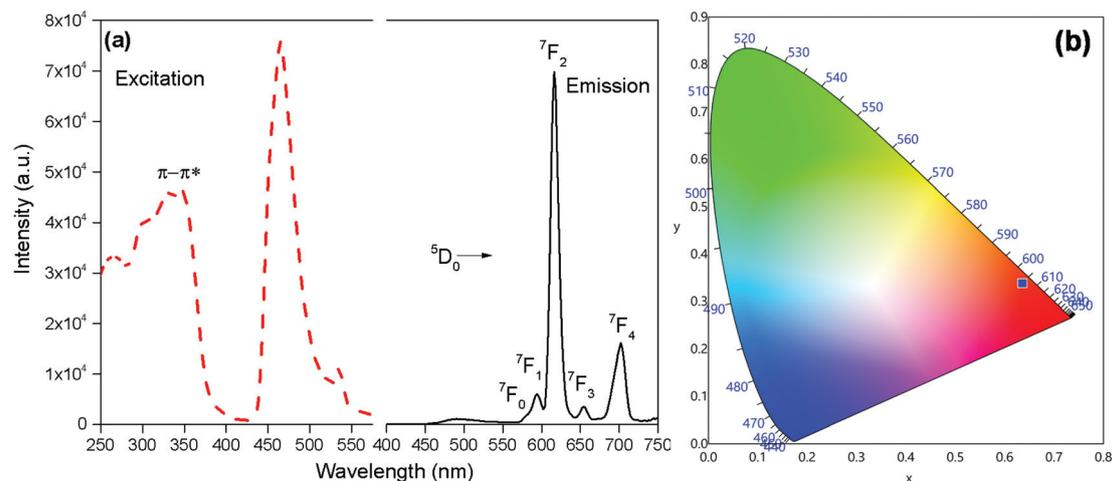
**Fig. 4** (a) Excitation (broken line) and emission (solid line) spectra ( $\lambda_{\text{ex}} = 345$  nm) (b) CIE-1931 chromaticity diagram demonstrating the calculated colour coordinate ( $x, y$ ) values for **[Eu(btfa)<sub>3</sub>1c]** in DCM at RT.
