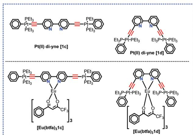
**Chart 1** Structure of the present and previously<sup>4c</sup> designed Pt(II) di-yne organometallic chromophore and their heterotrinnuclear (d–f–d) complex.
