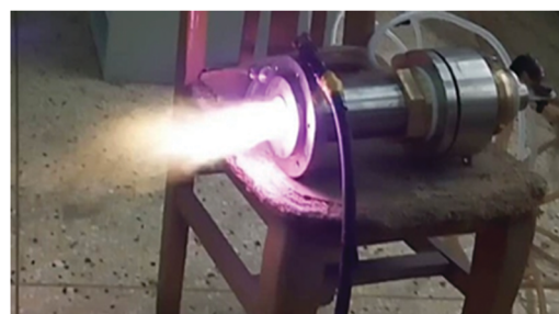
Fig. 9 Photograph of a 100 kW atmospheric thermal arc source in operation in the lab of the authors.
