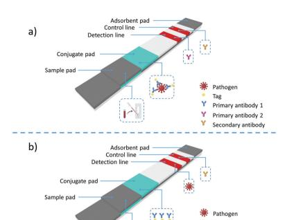
Fig. 2 Structure of a lateral-flow assay and the two main types of LFA formats: (a) sandwich format and (b) competitive format.
