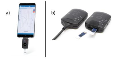
Fig. 17 (a) SenSit-smart miniaturized potentiostat connected to a mobile phone, and (b) Sensit-bt miniaturized wireless potentiostat developed by PalmSens (images from http://www.palmsens.com).
