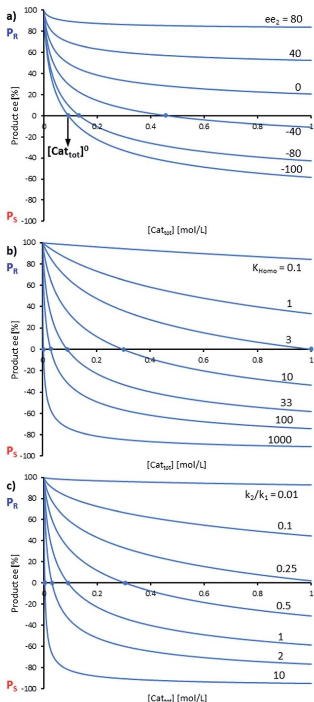
Fig. 5 Simulation of the relationship between  $ee_p$  and  $[Cat_{tot}]$  according to eqn (1) and (2). The basic set of parameters is  $ee_1 = 100$ ,  $ee_2 = -100$ ,  $K_{Homo} = 33$  and  $k_2/k_1 = 1$ . Each panel shows curves where one of the parameters has been varied: (a)  $ee_2$ , (b)  $K_{Homo}$ , (c)  $k_2/k_1$ . The product ee is defined as  $(P_R - P_S)/(P_R + P_S)$ .
