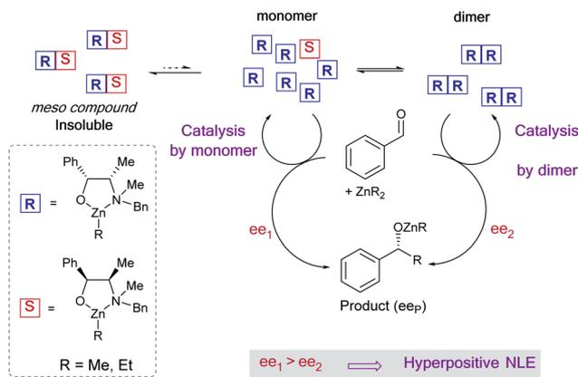
Fig. 1 Competitive reaction pathway of a monomeric and a dimeric catalyst in an enantioselective reaction that accounts for a hyperpositive non-linear effect: the case of NBE-catalysed enantioselective addition of dialkylzinc to benzaldehyde.
