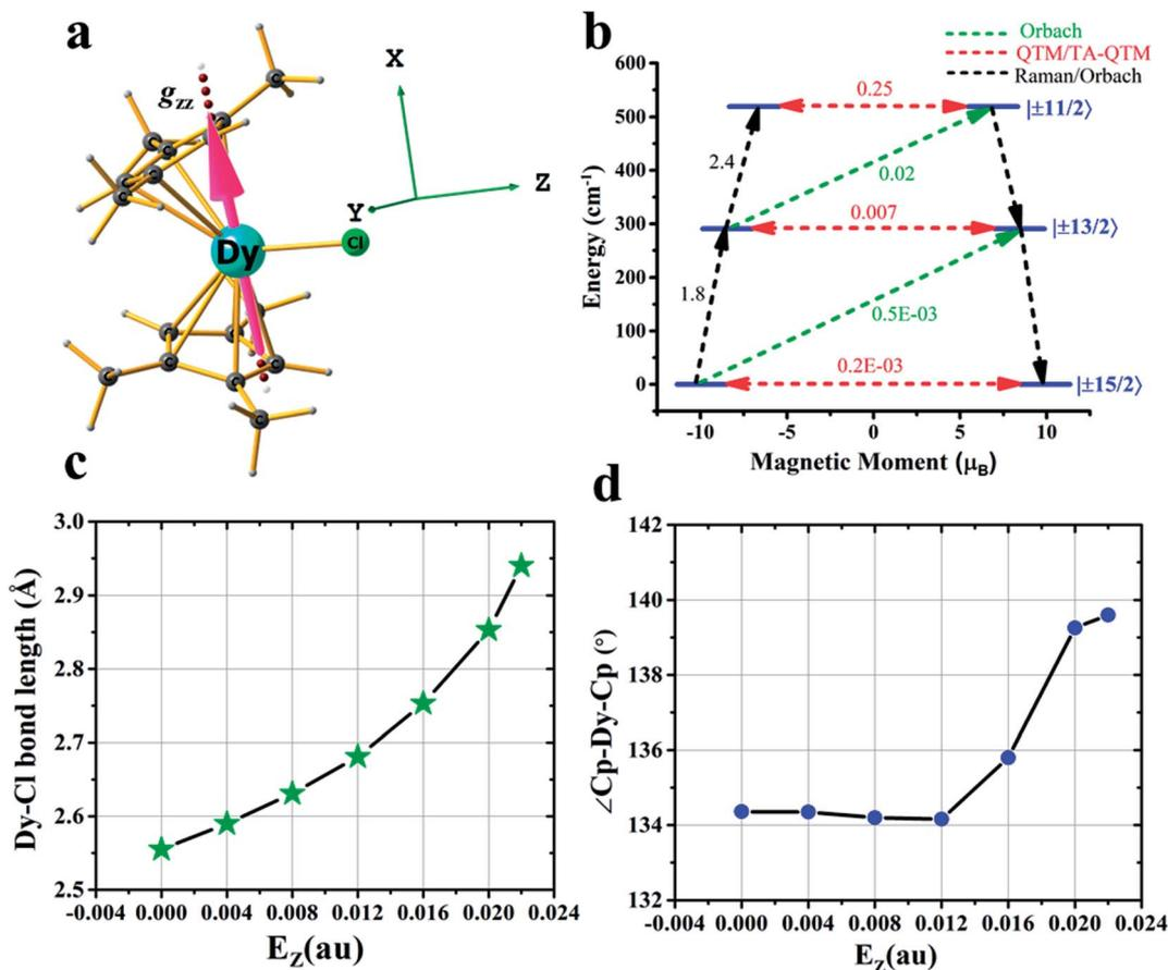
Fig. 3 Details of the application of an external electric field in complex 3. (a) DFT optimised geometry of complex 3, along with the  $g_{zz}$  axis and the three cartesian axes directions. (b) An *ab initio* computed magnetization blocking barrier diagram of  $^{22z}3_{\text{opt}}$ . See Fig. 1 caption for further details. (c) Variations in the Dy–Cl bond length and (d) Cp–Dy–Cp angle with respect to the oriented external electric field.
