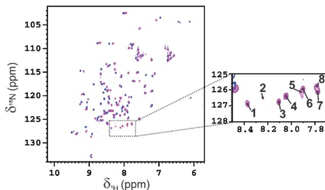
Fig. 5 2D  $^1\text{H}$ - $^{15}\text{N}$  HSQC spectra of WT-Ub (blue) and WT-Ub functionalized with the fucosyl derivative 7 on the Lys sidechains (**Fuc-Ub**, magenta) acquired at 298 K and 700 MHz. The signals in the area, selected by the dashed lines (enlarged on the right), correspond to the new amide groups obtained by the conjugation of the  $\epsilon$ - $\text{NH}_2$  group of lysine sidechains and the N-terminus with fucoside 7.
