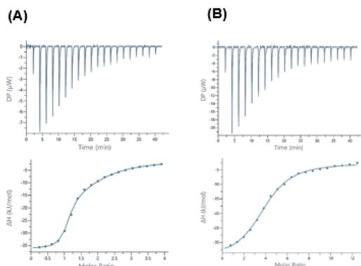
**Fig. 2** (A) Thermograms (top) and titration curves (bottom) obtained from the titration of (A) BamBL (50 μM) and (B) AFL (50 μM) by compound **3** (both 3 mM). Fitting procedure was performed using a two-site model for BamBL and with a one site model for AFL.
