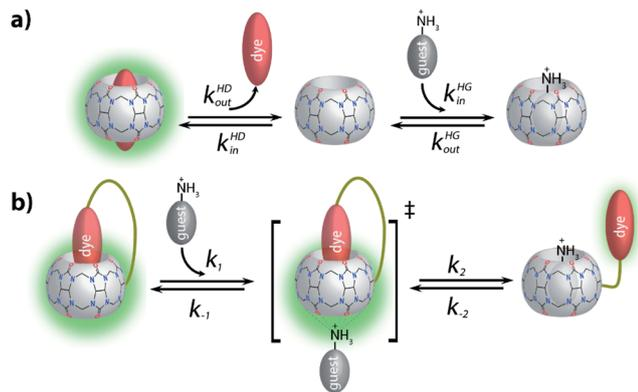
Fig. 9 (a) Schematic representation of a  $S_N1$ -type-mechanism for the guest-exchange process on analyte-induced conformational changes of non-covalent  $CB7 \supset$  dye reporter pair complexes; (b) schematic representation of a  $S_N2$ -type-mechanism for the guest-exchange process on analyte-induced conformational changes of  $CB7$ -dye conjugates.
