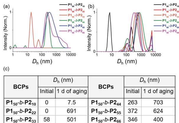
Fig. 1 DLS profiles of BCPs solutions (1 g L<sup>-1</sup> chloroform) (a) without aging and (b) after 1 day of aging at 25 °C. (c) A table of  $D_h$  values of the DLS profiles in (a) and (b).
