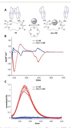
Fig. 12 (A) Model for reversible switching; (B) reversible ECD of (+)-1d and  $[Na\cdot(+)-1d]^+$  over 6 cycles; (C) reversible CPL of (-)-1d and  $[Na\cdot(-)-1d]^+$  over 6 cycles. Reproduced from ref. 23 with permission from the Royal Society of Chemistry.
