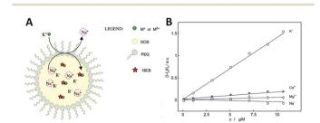
Fig. 10 (A) Ion-selective reverse micelles; (B) normalized fluorescence (406 nm) as a function of concentrations of different cations for 1d. Reproduced from ref. 8 with permission from the Royal Society of Chemistry.
