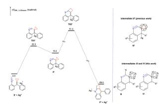
Fig. 1 DFT calculation on the reaction pathway via the ionic mechanism of previous work (relative Gibbs energy values in 1,4-dioxane solution are given in kcal mol<sup>-1</sup>).
