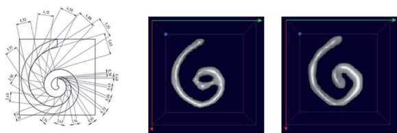
Fig. 7 Spiral phantom geometry (left) and MPI images of the phantom filled with 200 \mu\text{L} volume 15 mM iron concentration of T2 (30 nm) (right) and Resovist® (middle). The channel width of the phantom was 2 mm.
