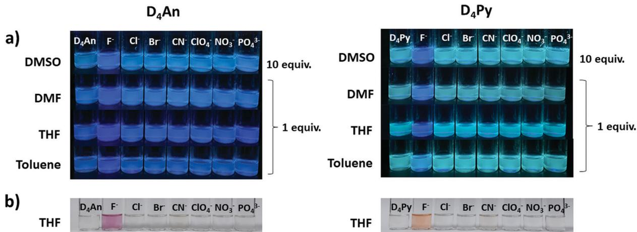
Fig. 3 Selective images of (a)  $D_4An$  ( $2 \times 10^{-5}$  M) (left) and  $D_4Py$  ( $1 \times 10^{-5}$  M) (right) after the addition of anions (1 and 10 equiv.) in various solvents under a UV lamp; (b)  $D_4An$  ( $4 \times 10^{-5}$  M) (left) and  $D_4Py$  ( $2 \times 10^{-5}$  M) (right) in THF upon the addition of anions (200 equiv.) under daylight.
