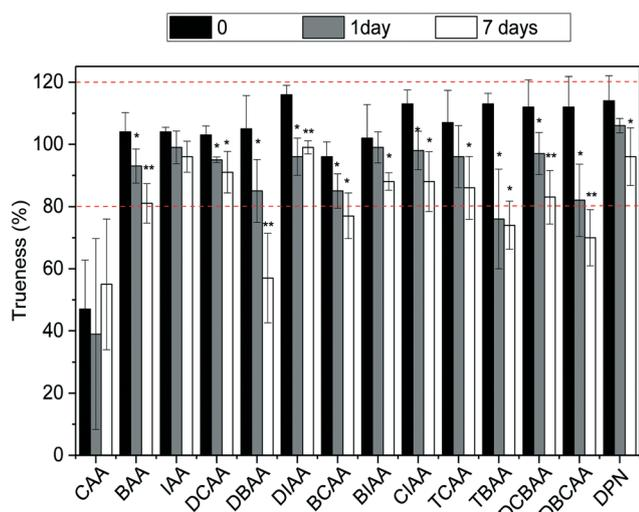
Fig. 3 Trueness values of HAAs and dalapon in tap water fortified at a concentration of  $5 \mu\text{g L}^{-1}$  and stored at  $-20 \text{ }^\circ\text{C}$  for 7 days. Error bars indicate RSD values of  $n = 3$  measurements.
