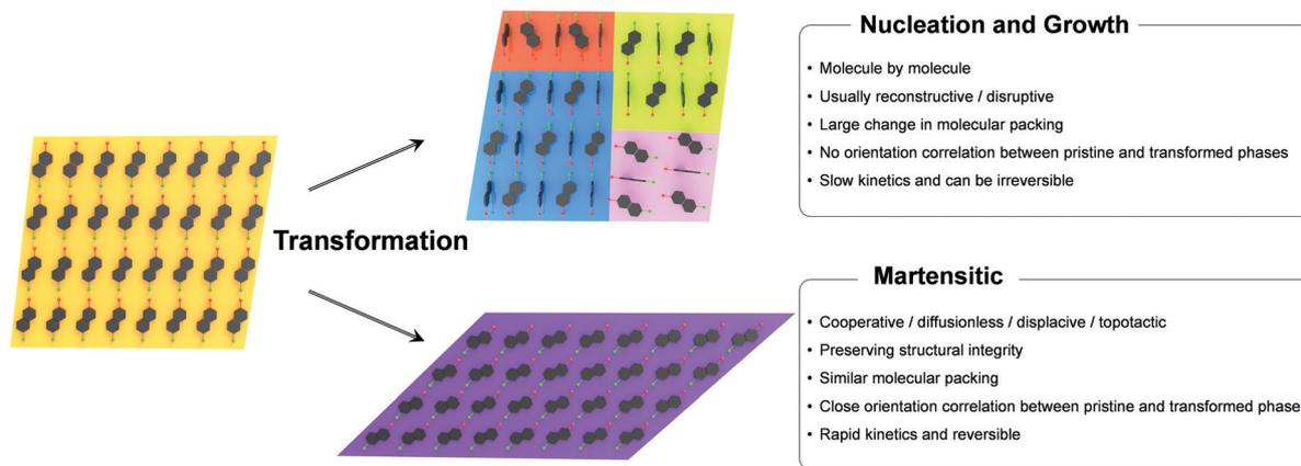
Fig. 3 General characteristics found in the nucleation and growth and martensitic transitions.
