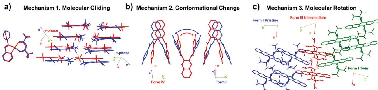
Fig. 6 Molecular mechanisms found in martensitic transitions, showing (a) molecular gliding,<sup>40</sup> (b) conformational change,<sup>46</sup> and (c) molecular rotation.<sup>57</sup> Examples of each mechanism are depicted by structural changes in #5 (CCDC 103651 and 1013657), #8 (CCDC 1583404 and 1583405), and #13 crystals (CCDC 1970910 and 1991343) of Fig. 2, respectively.
